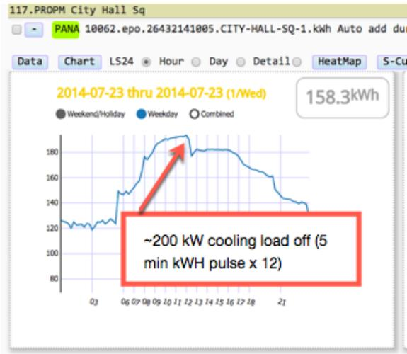
Figure 2. Discrete ~200kW load turning off.
