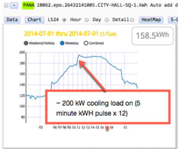
Figure 1. Discrete ~200kW load turning on.
